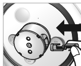
In Case of Improper Assembly of the One-Touch Button
