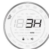
When the reheat finishes with the beep sound, keep warming function will be operated and show the time elapsed.
