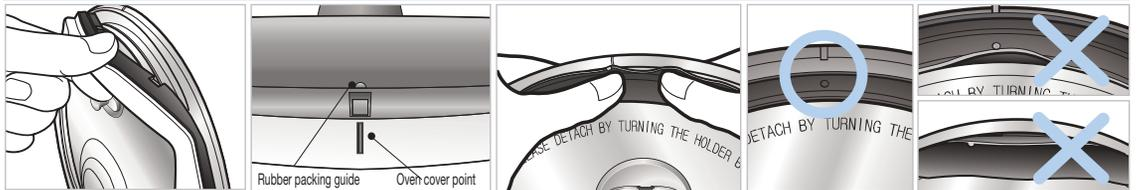
① To separate the rubber packing, please pull it out from the cover plate as shown in the picture.
