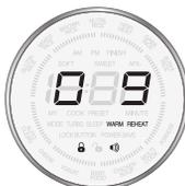
The lamp blinks and "9" indicator will show the reheat remaining time displayed in minutes with the mark going around clockwise.
